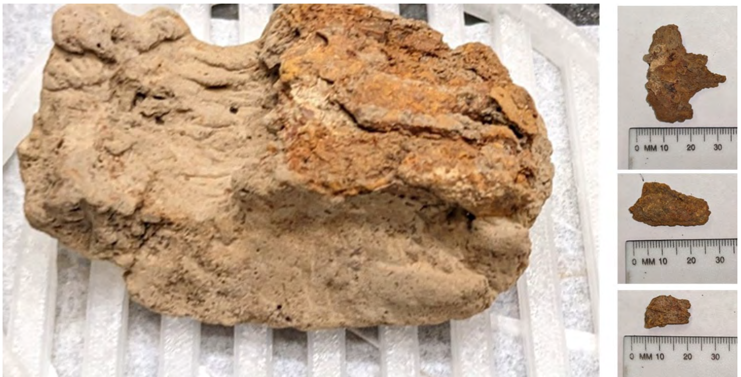
Figure 4. Photos of sediment rich specimen before (left) and after (right images) exposure to the electrolyte solution.
