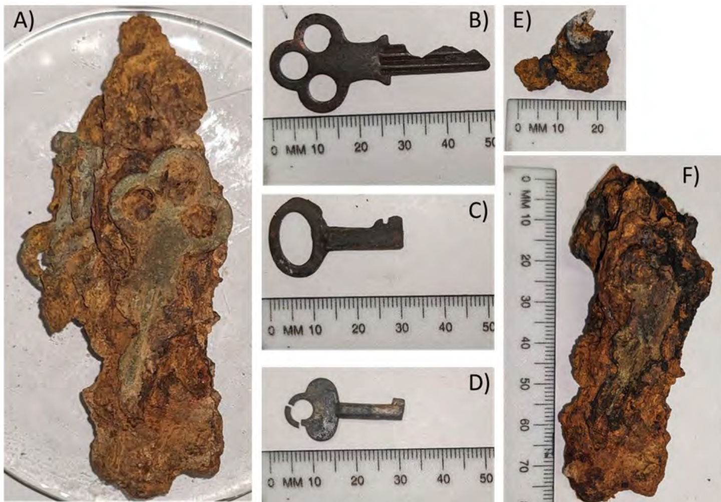
Figure 2. Photographs of the bulk keys specimens A) before electrolysis treatment and B-F) after electrolysis treatment.
