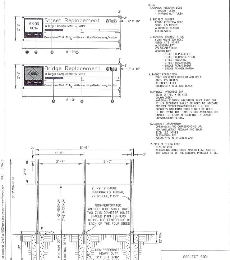
ASSEMBLY OF PLYWOOD SIGN
