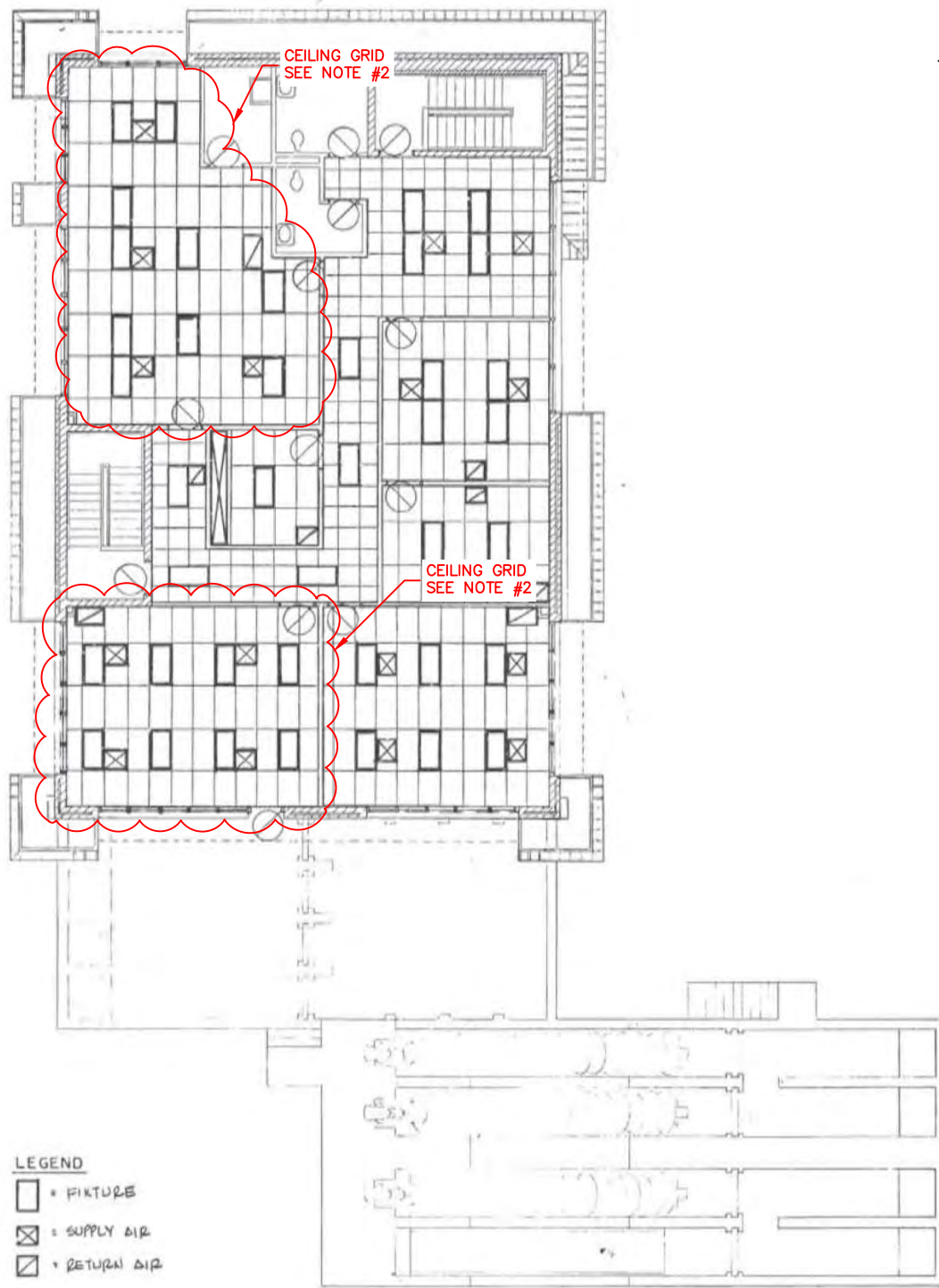
2 13 PLAN @ OPERATIONS BUILDING SECOND FLOOR PLAN REFLECTED CEILING SCALE: 1/8" = 1'-0"
