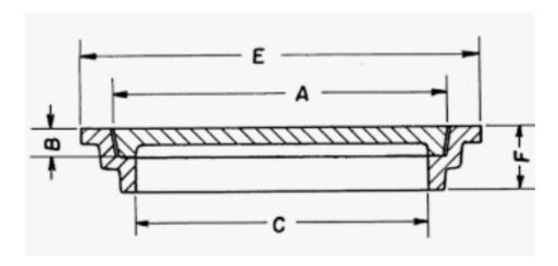
Where requested manhole frames and lids shall be Neenah model R6660-KH or equal and conform to the following dimensions:
