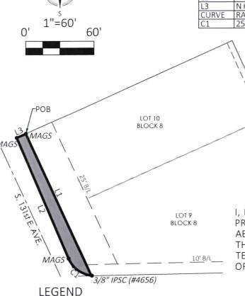
VACATION RIGHT OF WAY LINE TABLE LINE BEARING DISTANCE S 23°18'58" E 138.51 L1 N 21°47'30" W 116.62 N 66°41'02" 8.74 RADIUS ARC LENGTH CHORD LENGTH CHORD BEARING DELTA ANGLE N 51°41'16" W 59°47'33" 25.00' 26.09' 24.92
